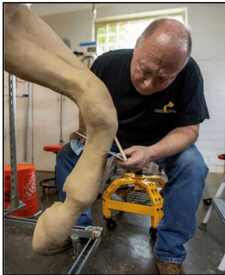
Tommy Ladd, owner of Schaefer Art Bronze Casting, uses playing cards to mark the areas where the statue will be cut and molded. The statue is taken apart before being cast in bronze at the foundry. (Brad Tollefson/The Washington Post)
